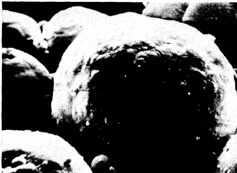
FIG. 1. The unused copper powder, as supplied; \times 1300 .
